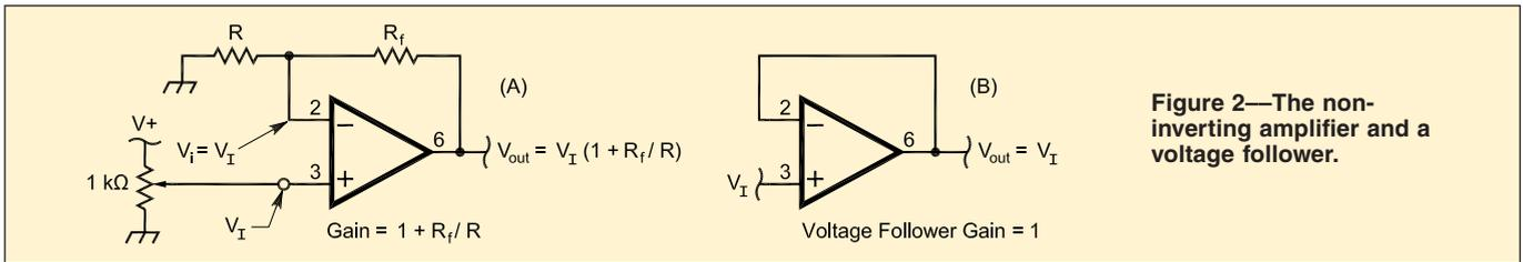
Figure 2—The non-inverting amplifier and a voltage follower.
